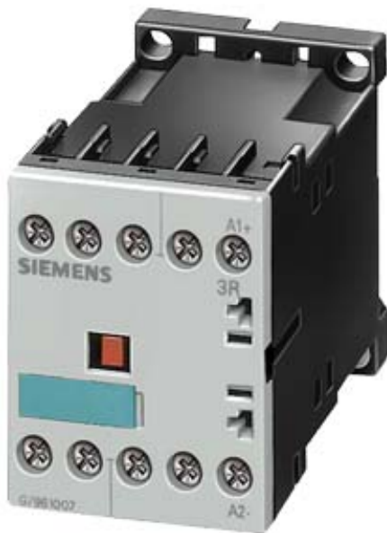
COUPLING RELAY, AC-3 4 KW/400 V, 1 NC, DC 24 V, 0.7...1.25*US, W. VARISTOR, 3-POLE, SIZE S00, SCREW CONNECTION
