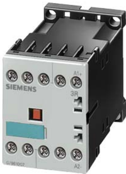
CONTROL RELAY, AC-3 4 KW/400 V, 1 NC, 110 V DC, 0.7...1.25*US, W.VARISTOR, 3-POLE, SIZE S00, SCREW CONNECTION
