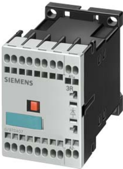
COUPLING RELAY, AC-3 4 KW/400 V, 1 NO, DC 24 V, 0.7...1.25*US, 3-POLE, SIZE S00, CAGE CLAMP CONNECTION
