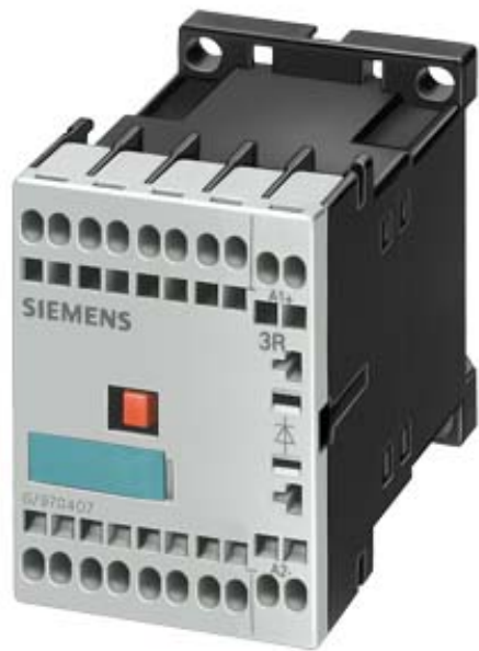
COUPLING RELAY, AC-3 5,5KW/400 V, 1 NO, DC 24 V, 0.7...1.25*US, 3-POLE, SIZE S00, CAGE CLAMP CONNECTION
