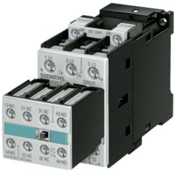
CONTACTOR, AC-3 4 KW/400 V, DC 220 V, 3-POLE, 2 NO + 2 NC, SIZE S0, SCREW CONNECTION
