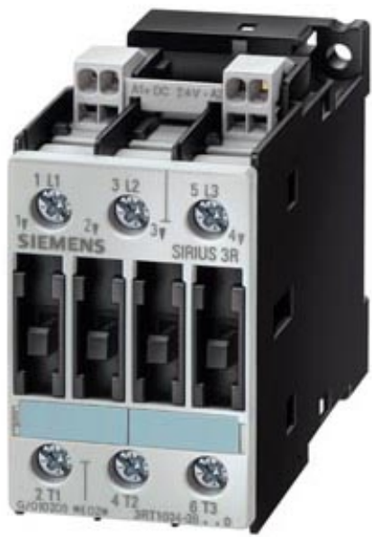
CONTACTOR, AC-3 4KW/400V, AC 220V, 50/60 HZ 3-POLE, SIZE S0, CAGE CLAMP CONNECTION
