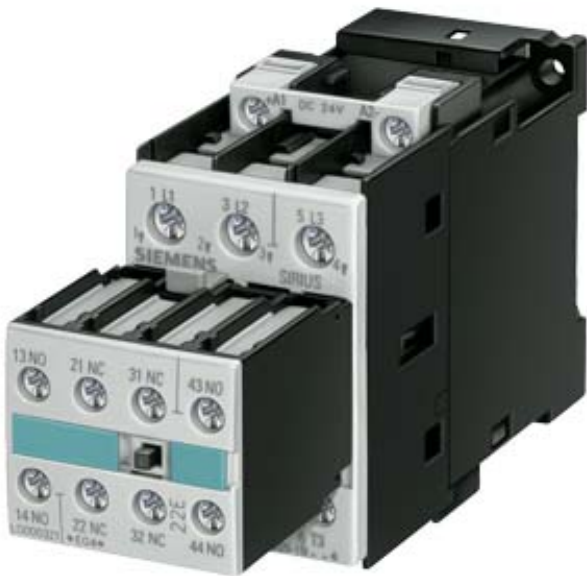
CONTACTOR, AC-3 5.5 KW/400 V, AC 24 V, 50 HZ, 3-POLE, 2 NO + 2 NC, SIZE S0, SCREW CONNECTION
