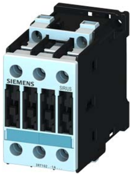
CONTACTOR, AC-3 5.5 KW/400 V, AC 24 V, 50/60 HZ, 3-POLE, SIZE S0, SCREW CONNECTION
