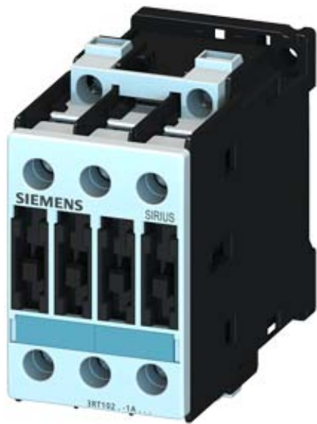
CONTACTOR, AC-3 5,5 KW/400 V, AC 480 V, 60 HZ, 3-POLE, SIZE S0, SCREW CONNECTION
