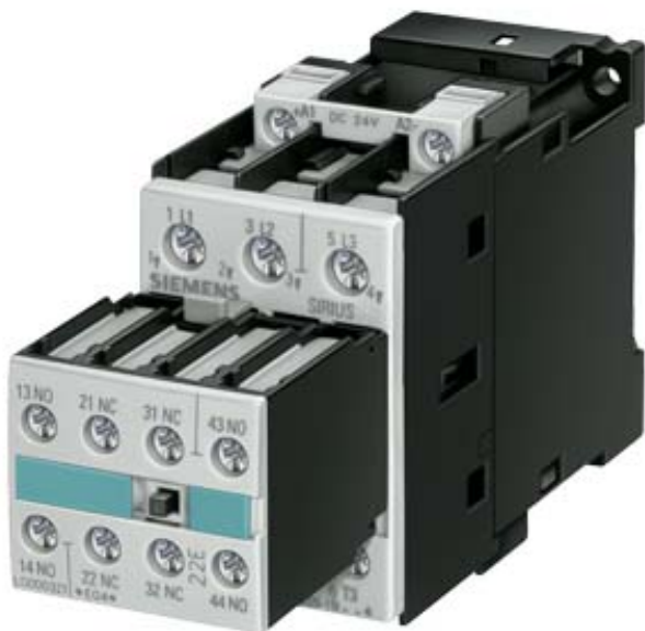
CONTACTOR, AC-3 5.5 KW/400 V, DC 60 V, 3-POLE, 2 NO + 2 NC, SIZE S0, SCREW CONNECTION
