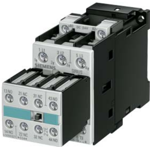
CONTACTOR, AC-3 5.5 KW/400 V, DC 125 V, 3-POLE, 2 NO + 2 NC, SIZE S0, SCREW CONNECTION
