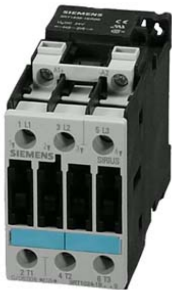
CONTACTOR 3-PH 5.5 KW/400 V, 24 V DC, 0.7...1.25*US, WITH VARISTOR, 3-POLE, SIZE S0, SCREW CONNECTION STANDING MOUNTING POSITION
