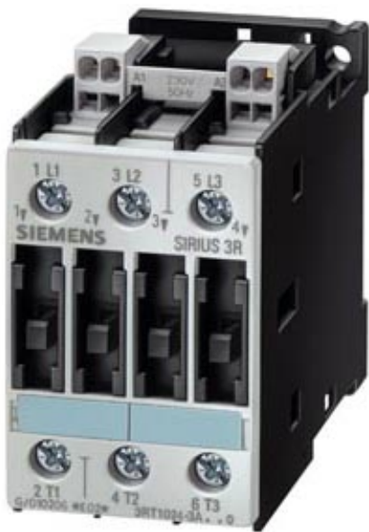
AC-3 CONTACTOR, 5.5 KW/400 V, 277 V, 60 HZ AC 3-POLE, SIZE S0 CAGE CLAMP CONNECTION
