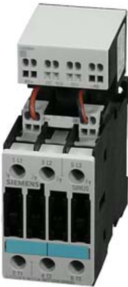
CONTACTOR, AC-3 5,5 KW/400 V, AC110V 50/60HZ 3-POLE, SIZE S0, SCREW CONNECTION
