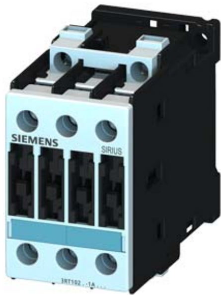
CONTACTOR 3-PH 7.5 KW/400 V, 24 V AC 60 HZ 3 -POLE, SIZE S0, SCREW CONNECTION
