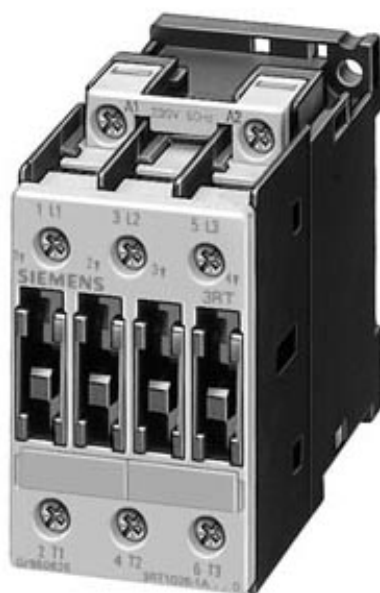
CONTACTOR, AC-3 7.5 KW/400 V, DC 42 V, 3-POLE, SIZE S0, SCREW CONNECTION
