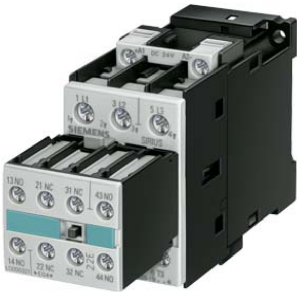
CONTACTOR, AC-3 7.5 KW/400 V, DC 42 V, 3-POLE, 2 NO + 2 NC, SIZE S0, SCREW CONNECTION
