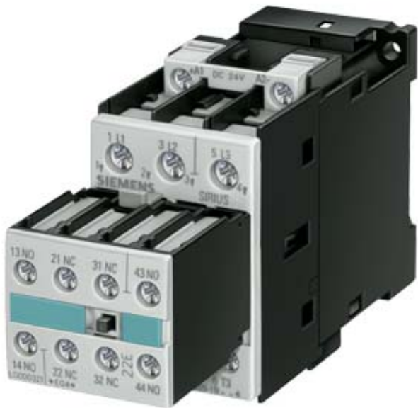
CONTACTOR, AC-3 7.5 KW/400 V, DC 220 V, 3-POLE, 2 NO + 2 NC, SIZE S0, SCREW CONNECTION
