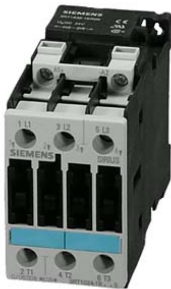
CONTACTOR 3-PH 7.5 KW/400 V, 24 V DC, 0.7...1.25*US, WITH VARISTOR, 3-POLE, SIZE S0, SCREW CONNECTION STANDING MOUNTING POSITION
