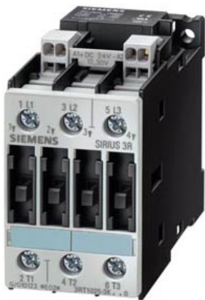
CONTACTOR, AC-3 7,5 KW/400 V, AC 220 V 50 HZ/ 240 V 60 HZ, 3-POLE, SIZE S0, CAGE CLAMP CONNECTION
