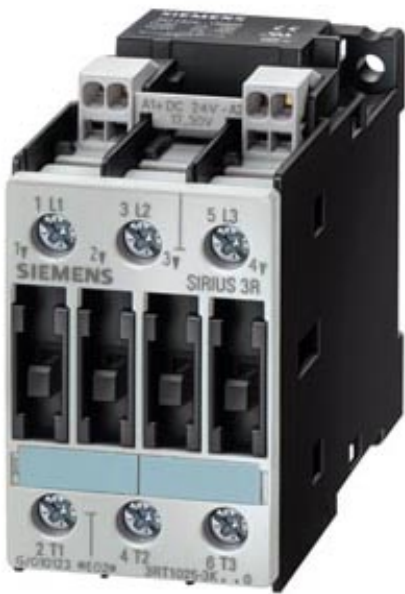
CONTACTOR, AC-3 7.5 KW/400 V, DC 24 V, 3-POLE, SIZE S0, CAGE CLAMP CONNECTION
