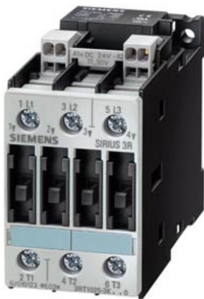
CONTACTOR, AC-3 7.5 KW/400 V, DC 42V, 3-POLE, SIZE S0, CAGE CLAMP CONNECTION
