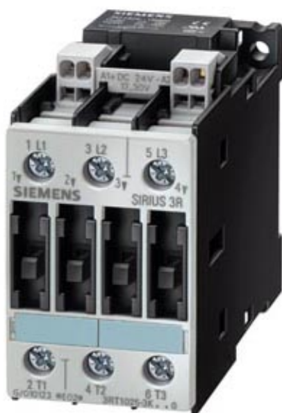
CONTACTOR, AC-3 7.5 KW/400 V, DC 110 V, 3-POLE, SIZE S0, CAGE CLAMP CONNECTION
