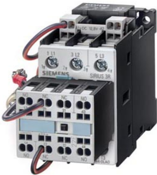
CONTACTOR, AC-3 7.5KW/400V, DC 24V, 0.7...1.25*US, 3-POLE, SIZE S0, CAGE CLAMP CONNECTION
