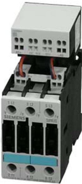
CONTACTOR, AC-3, 7.5KW/400V DC 110V,0.7...1.25*US,3-POLE SIZE S0, CAGE CLAMP CONNECTION WITH SOLID-STATE CONTROL BLOCK VARISTOR INTEGRATED
