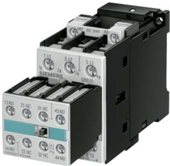
CONTACTOR, AC-3 11 KW / 400 V, AC 230 V 50/60 HZ, 3-POLE, 2 NO + 2 NC, SIZE S0, SCREW CONNECTION
