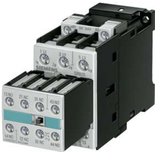
CONTACTOR, AC-3 11 KW/400 V, AC 230 V, 50 HZ, 3-POLE, 2 NO + 2 NC, SIZE S0, SCREW CONNECTION
