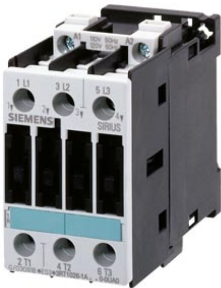
CONTACTOR, 10HP 460/575V DC 24V 3-POLE, SIZE S0 SCREW CONNECTION NEMA SIZE 1
