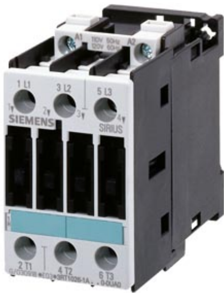
CONTACTOR, AC-3 11 KW/400 V, DC 125 V, 3-POLE, SIZE S0, SCREW CONNECTION, MOUNTING POSITION VERTICAL
