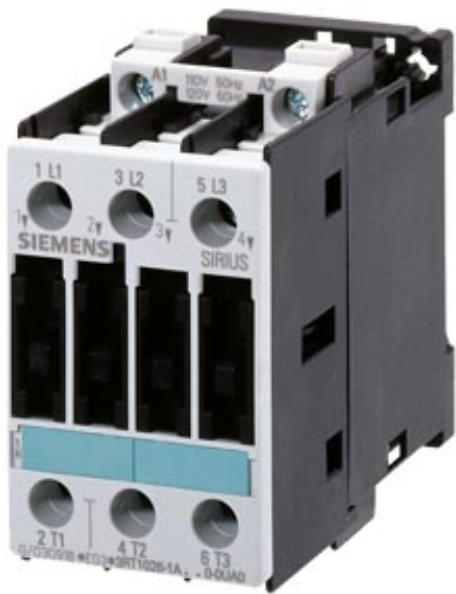
CONTACTOR, AC-3 11 KW/400 V, DC 48 V, 3-POLE, SIZE S0, SCREW CONNECTION
