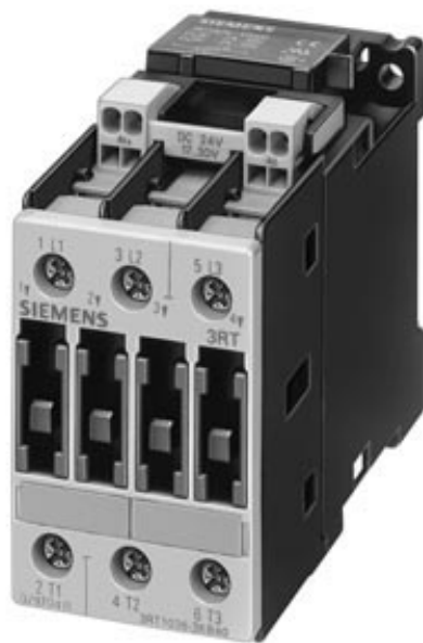
CONTACTOR, AC-3 11 KW/400 V, AC 24 V 50/60 HZ, 3-POLE, SIZE S0, CAGE CLAMP
