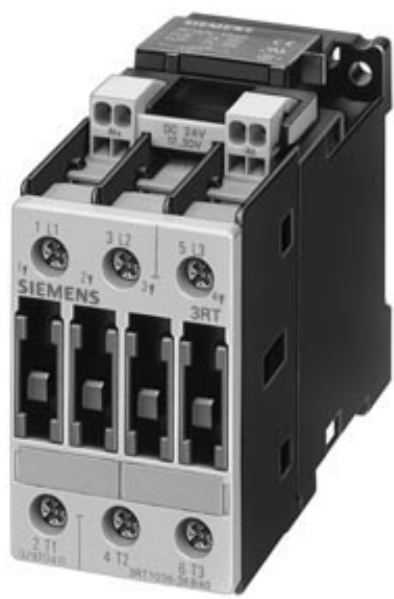
CONTACTOR, AC-3 11 KW/400 V, AC 110 V, 50 HZ, 3-POLE, SIZE S0, CAGE CLAMP
