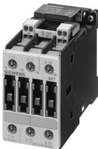
CONTACTOR, AC-3 11 KW / 400 V, AC 220 V 50/60 HZ, 3-POLE, SIZE S0, CAGE CLAMP
