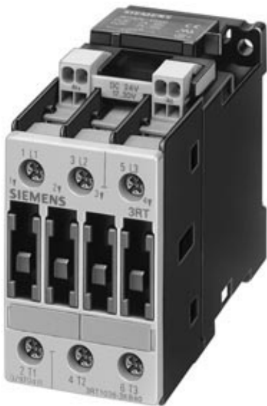
CONTACTOR, AC-3 11 KW/400 V, AC 230 V, 50 HZ, 3-POLE, SIZE S0, CAGE CLAMP
