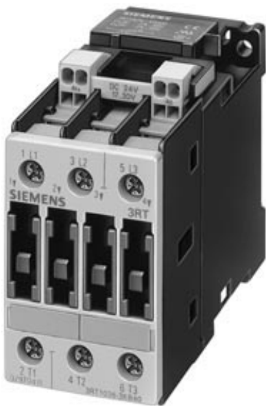
CONTACTOR, AC-3 11KW/400V, DC 24V, 0.7...1.25*US, 3-POLE, SIZE S0, CAGE CLAMP CONNECTION STANDING MOUNTING POSITION
