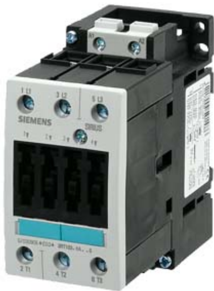
CONTACTOR, AC-3 15 KW/400 V, AC 24V 50/60HZ, 3-POLE, SIZE S2, SCREW CONNECTION
