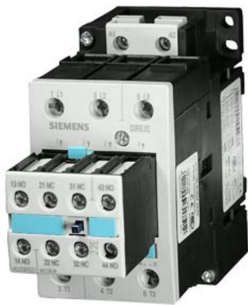
CONTACTOR, AC-3 15 KW/400 V, AC 220V 50HZ/240V 60HZ 2 NO + 2 NC 3-POLE, SIZE S2, SCREW CONNECTION
