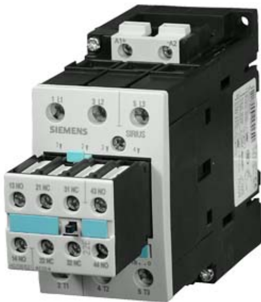
CONTACTOR, AC-3 15 KW/400 V, DC 220 V, 3-POLE, 2 NO + 2 NC, SIZE S2 SCREW CONNECTION
