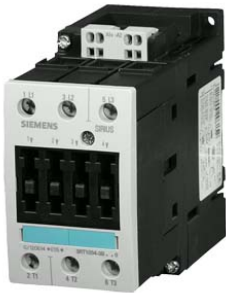
CONTACTOR, AC-3 15 KW/400 V, DC 110 V, 3-POLE, SIZE S2, CAGE CLAMP
