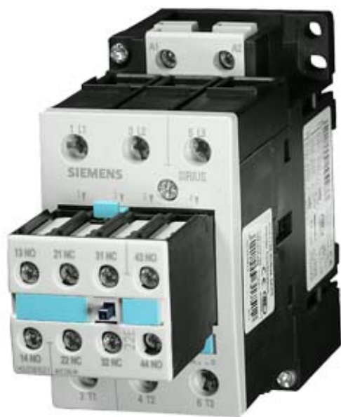
CONTACTOR, AC-3 18.5 KW/400 V, AC 24V 50/60HZ, 2 NO + 2 NC, 3-POLE, SIZE S2, SCREW CONNECTION
