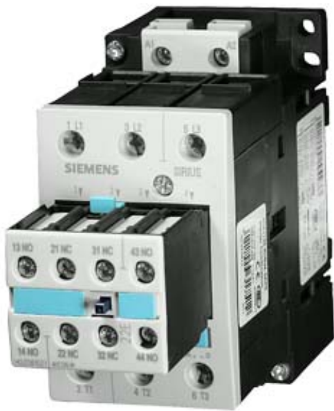
CONTACTOR, AC-3 18.5 KW/400 V, AC 48 V, 50 HZ, 2 NO + 2 NC, 3-POLE, SIZE S2, SCREW CONNECTION
