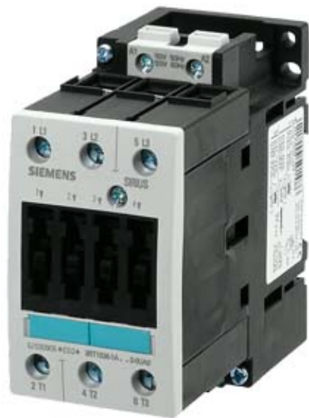
CONTACTOR, AC-3 18.5 KW/400 V, DC 24 V, 3-POLE, SIZE S2, SCREW CONNECTION
