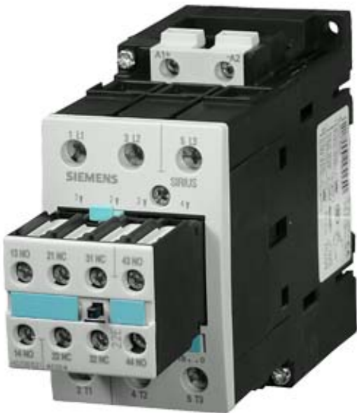
CONTACTOR, AC-3 18.5 KW/400 V, DC 42 V, 3-POLE, 2 NO + 2 NC, SIZE S2, SCREW CONNECTION
