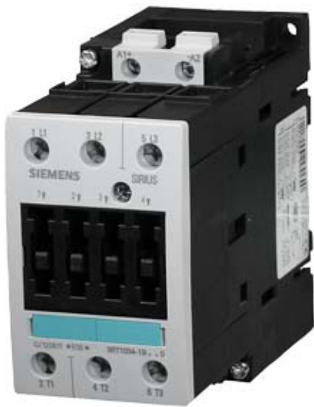
CONTACTOR, AC-3 18.5 KW/400 V, DC 230 V, 3-POLE, SIZE S2, SCREW CONNECTION
