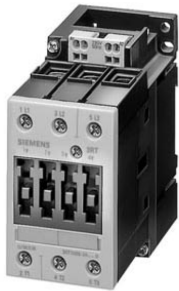
CONTACTOR, AC-3 18.5 KW/400 V, AC 230 V, 50 HZ, 3-POLE, SIZE S2, CAGE CLAMP
