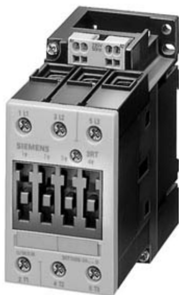
CONTACTOR, AC-3 18,5 KW/400 V, AC 220 V 50 HZ/ 240 V 60 HZ, 3-POLE, SIZE S2, CAGE CLAMP
