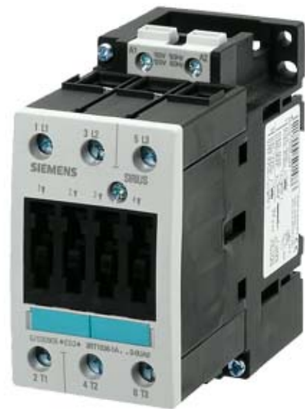
CONTACTOR, AC-3 22 KW/400 V, AC 24 V, 50 HZ, 3-POLE, SIZE S2, SCREW CONNECTION MOUNTING POSITION VERTICAL
