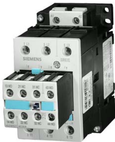
CONTACTOR, AC-3 22 KW/400 V, AC 24V 50/60HZ, 2 NO + 2 NC, 3-POLE, SIZE S2, SCREW CONNECTION
