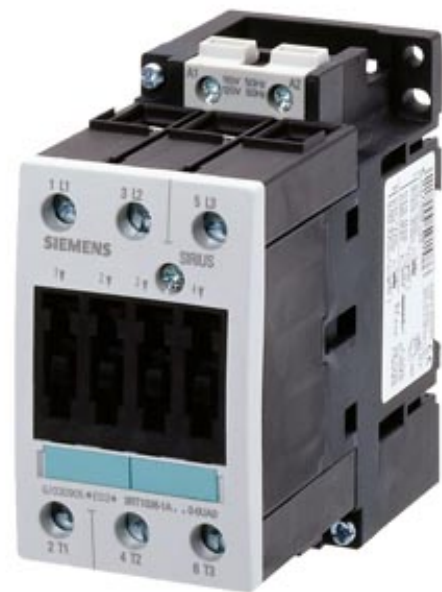
CONTACTOR, AC-3 22 KW/400 V, AC 110 V, 50 HZ, 3-POLE, SIZE S2, SCREW CONNECTION MOUNTING POSITION VERTICAL
