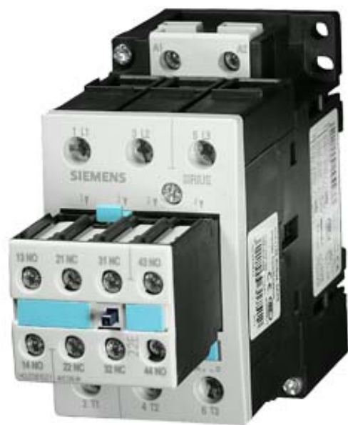
CONTACTOR, AC-3 22 KW/400 V, AC 110V 50/60HZ, 2 NO + 2 NC, 3-POLE, SIZE S2, SCREW CONNECTION
